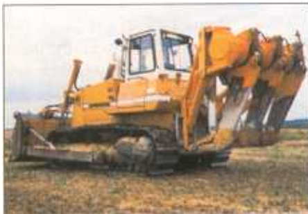
Special machines for special problems - chisel stroke loosening machine combining two different operations
